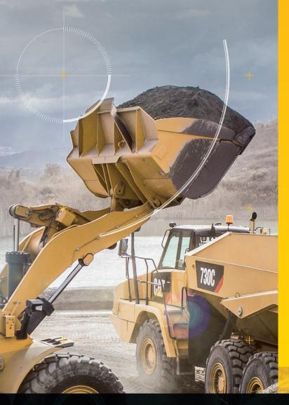
**CAT® PAYLOAD** is an integrated weighing technology that displays the weight of the bucket in the cab, allowing operators to fill trucks correctly the 1st time.
